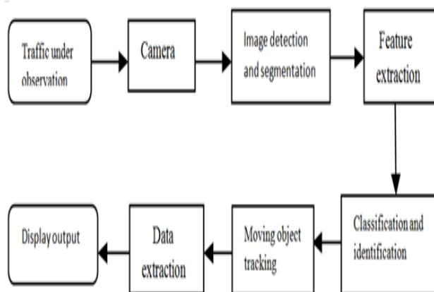
Fig 1. A Vehicle Analysis System in Typical Video [39]
